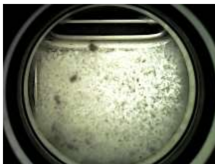
Figure 1. Solid-liquid-liquid-vapor Q-point for carbon dioxide + o -terphenyl binary system at 294.57 K and 5.21 MPa with 61,10 mol% CO 2 .
